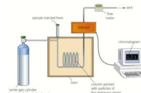
Figure 4 The metal column in gas chromatography is coiled so that it can fit into a very hot oven.
