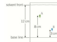
Figure 3 A thin-layer chromatogram for substances A and B.
