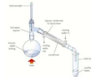
Fractional distillation two or more substances from a mixture in the liquid state. Each substance must have a different boiling point
