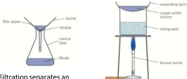
Filtration separates an insoluble solid from a liquid
