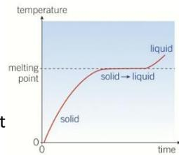
Figure 4 The temperature of a pure substance remains constant while it melts.
